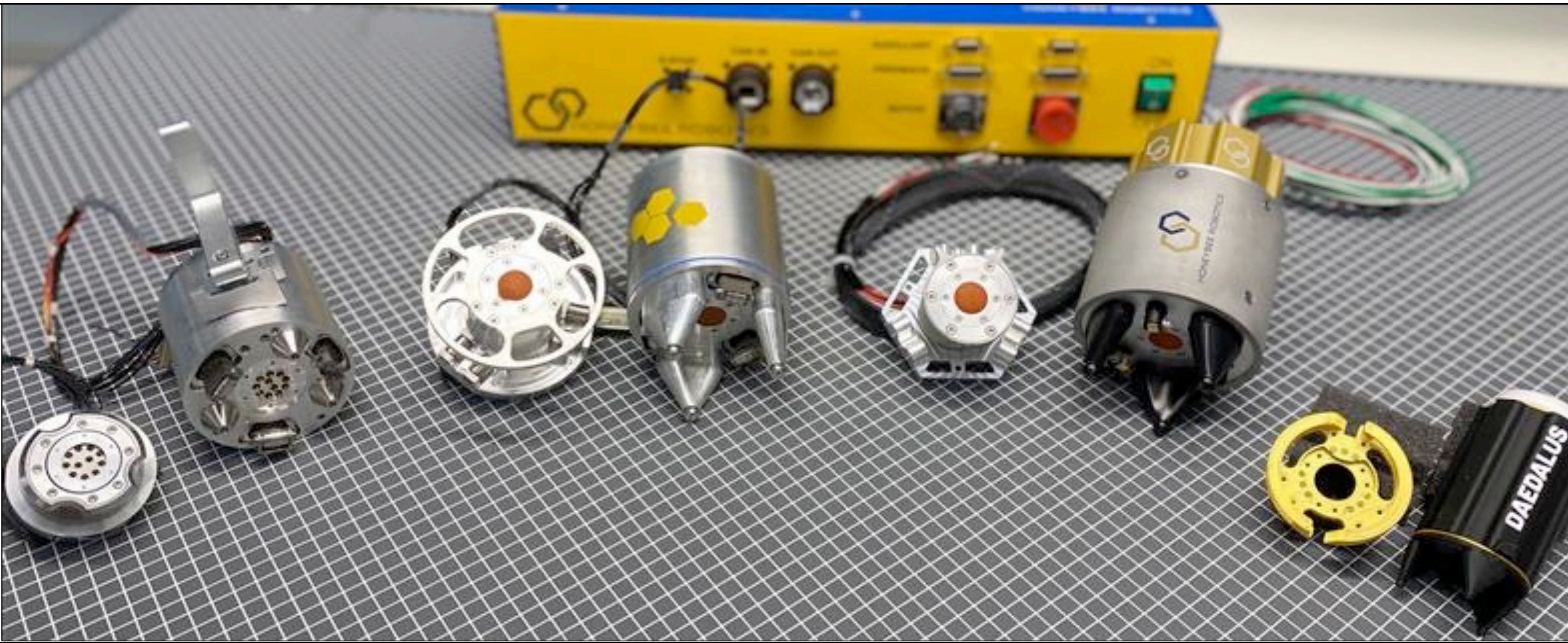
Figure 1. Honeybee Robotics Dust Tolerant Electrical Connector Lineage; Left to Right: c. 2011 Socket Unit & Manual Plug, c.2012 Socket and Motorized Plug, c.2023 Socket & Manual Plug, c.2024 A 3D Printed Prototype Of The Latest Socket and Manual Link Units
